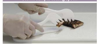
Spoon in moulded polycarbonate, indented and with 3 claws forming a fork. To cut sterile samples easily. Autoclavable at 121°C.
