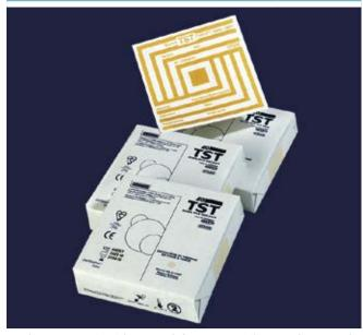
Ready-to-use Bowie-Dick test pack for steam sterilizers. Indicator to be used in specific tests as defined in EN 867-1 class B and 867-4 and ISO 11140 class 2. Instructions for use: place the test in the centre of the top shelf and perform a BD cycle. Open the packet and check the sheet: a successful test is blue, another colour indicates a failure.
