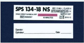
The Prion 134-18 NS emulator is a multi-parameter class 6 indicator (temperature, time and saturated steam). It is used for steam sterilisation, Prion cycle 134  $^{\circ}$ C / 18 minutes.
