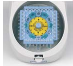
A single rotor for tubes and tube strips
