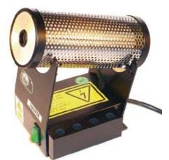
Sterilises loops for seeding, needles, culture tubes and small instruments effectively, destroying any organic material in 5/8 seconds at a temperature of 900 ° C.
